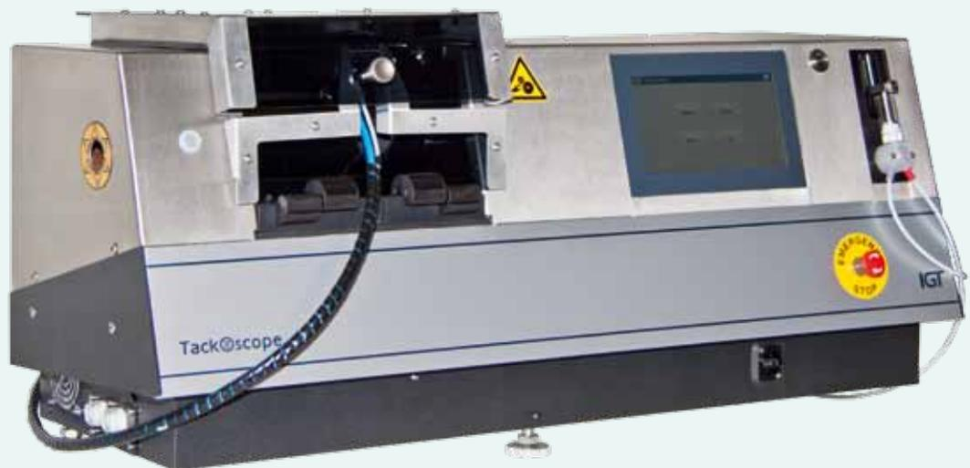
**Rheology measurements are a major factor in the development and production of printing inks, raw materials for inks and other pasty liquids. Important factors for offset printing inks are tack (or stickiness of the ink), water pick-up, water release and viscosity.**
