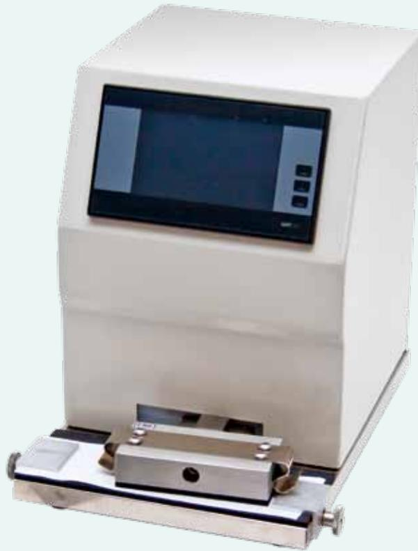
Rub resistance determines the suitability of printed matter, folding cartons, brochures, newspapers, and wrappers for further processing, mailing or other purposes. It is influenced by the properties and combinations of ink, substrate, spray powder, varnish and dampening liquid. Therefore, test of rub resistance is vital to printers, converters and manufacturers of inks and substrates.
