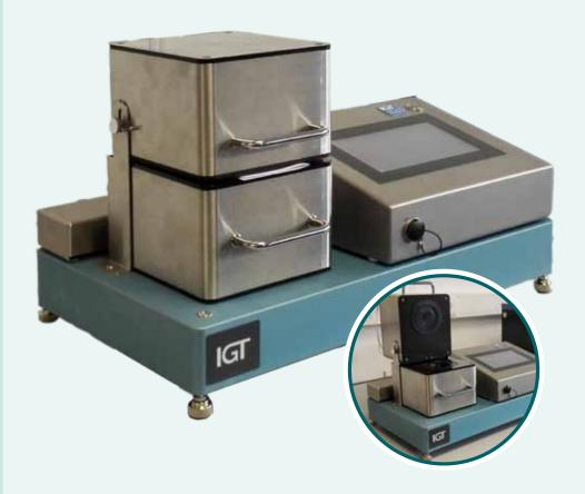
The IGT SizeOscope is an automated device to determine the sizing of paper and board through the change in reflectivity. It is especially designed to be used with watery liquids of all kinds, its materials coming in contact with the liquid are suitable for all usual liquids common in the paper industry.
